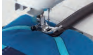
Thick handle can be sewn with ease. 3-12-3 layers of denim.
